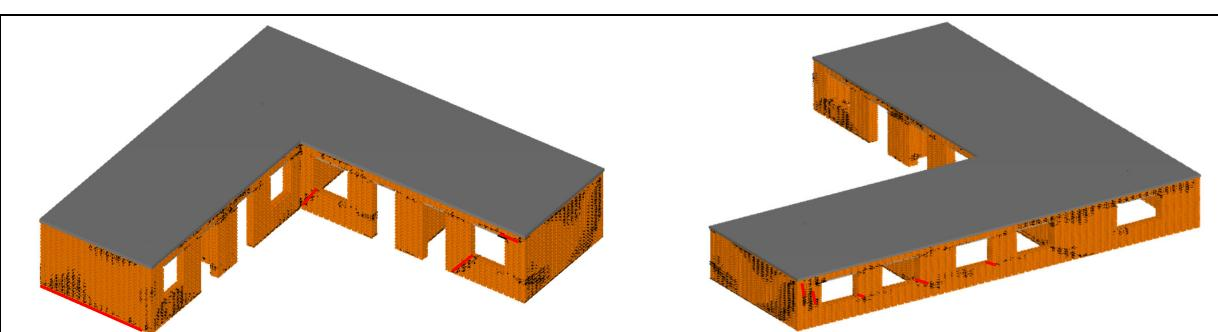
**CP Threshold:** Major cracks (black, shear and flexural) of average width 7 mm extended through all the wall surfaces. Several piers (mainly on the front side walls) developed shear cracks of width more than 12.5 mm and flexural cracks of opening more than 4 mm. A major horizontal crack (red) of 4 mm opening appeared in the solid IP walls.
