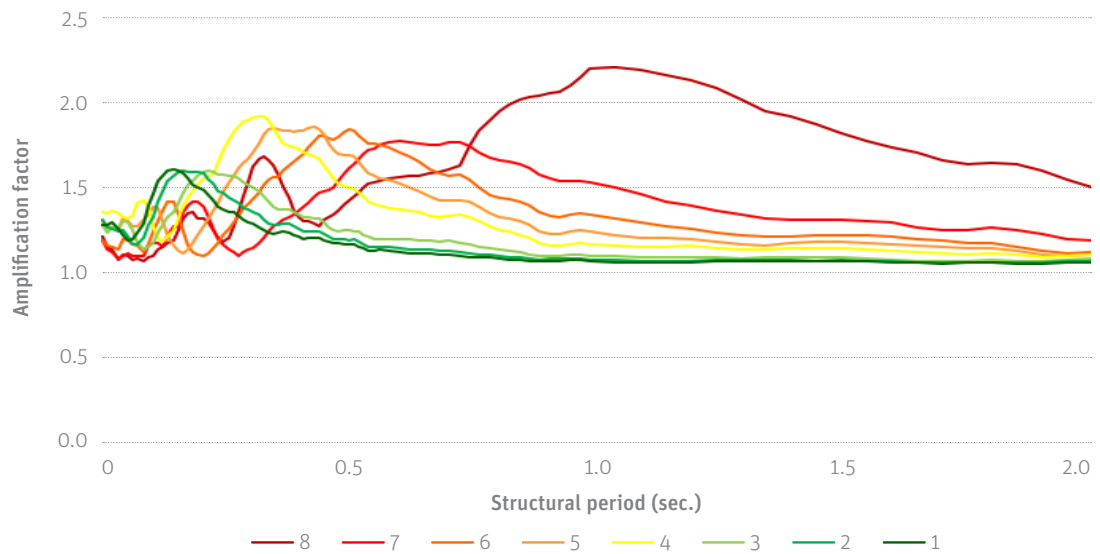
c) Final amplification spectra for the eight types of soil defined
