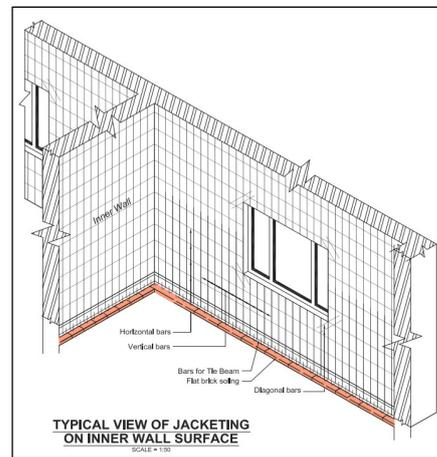
Inner surface reinforcement details
