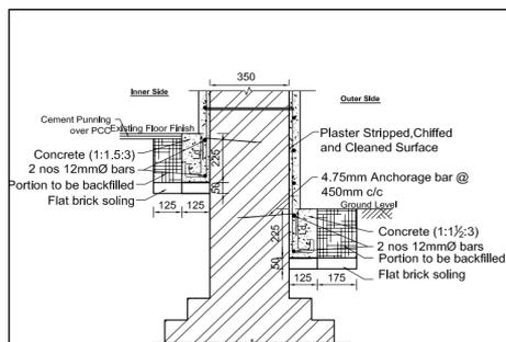
Cross sectional details of the foundation, reinforcement and plaster layer
