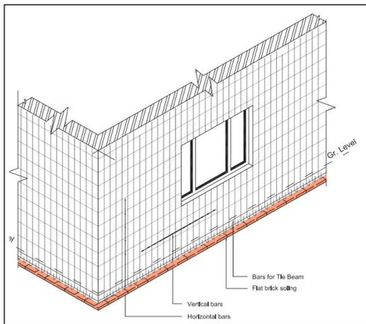
Outer surface reinforcement details
