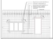
Details of reinforcements including the diagonal bars at the corners of openings.
