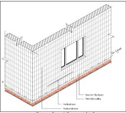
Outer surface reinforcement details
