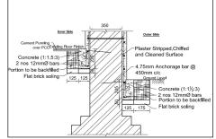
Cross sectional details of the foundation, reinforcement and plaster layer
