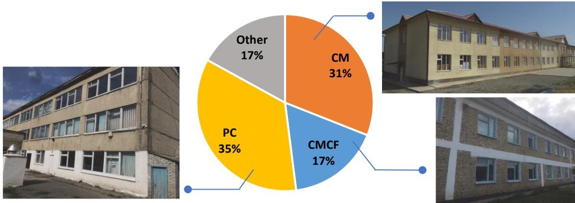
Figure 3: Distribution of common building types (long axis of the building) from field inspection of a subset of 78 eligible schools
