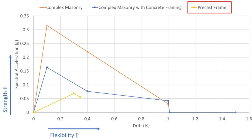
Figure 5: Representative pushover curve of the index buildings showing their original seismic capacity
