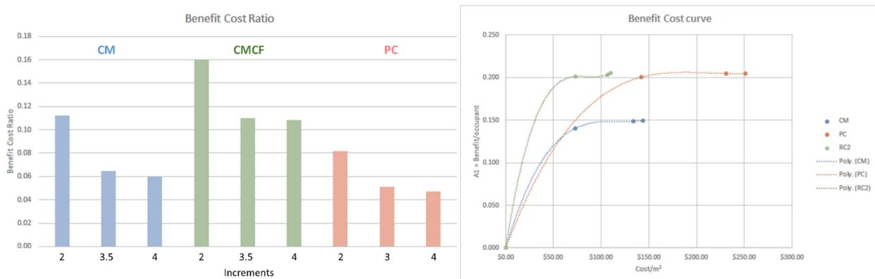
Figure 8: Benefit-cost of considered retrofit increments for 3 building types (left: benefit-cost ratio per increment; right: fitted curves demonstrating the relationship between the safety/benefit index and cost for seismic retrofit.)
