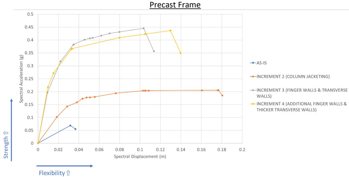
Figure 6: Capacity curves showing seismic capacity improvements for typical school building types
