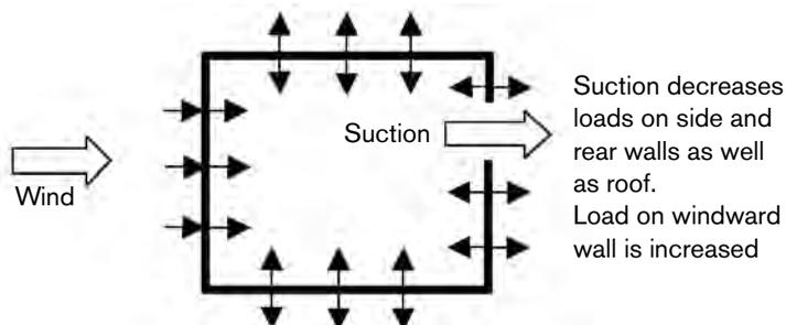
walls, rear wall and roof inward. This inward force counteracts the suction force of the wind outside the building. Therefore the load on the side and rear walls and on the roof are diminished.
