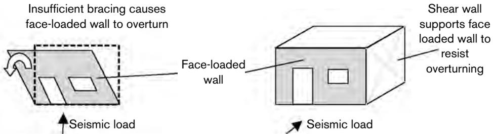
As shear walls help to brace face-loaded walls and stop them from overturning, the corners where they meet should be reinforced.
