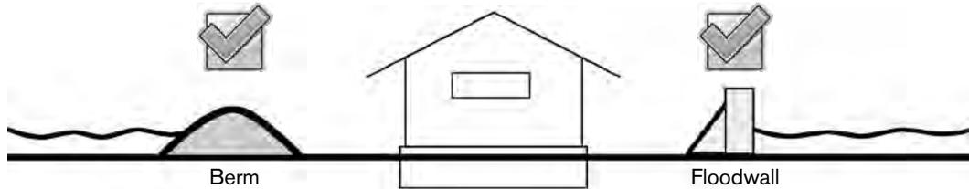
There are several different types of barriers commonly built to reduce flooding. Levees are commonly built along rivers and other bodies of water to prevent overflow. Berms, made of earth, and floodwalls, commonly made of concrete are built at the site. When considering flood barriers, it is essential to design systems for drainage if floodwaters overflow the barriers.
