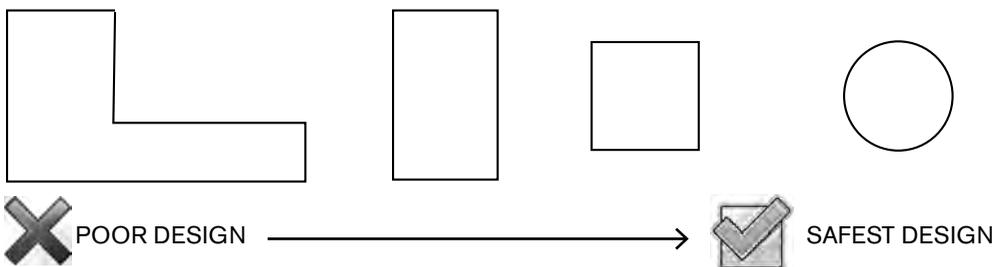
The asymmetry of structural elements can result in damaging ‘twisting’ forces. Structural layouts, such as U- and L-shaped buildings, amplify these twisting forces and their inside corners are particularly vulnerable to damage. These types of structures should be avoided. If such layouts are desired, it is preferable to design several distinct symmetrical buildings oriented in such a way as to produce similar results.
