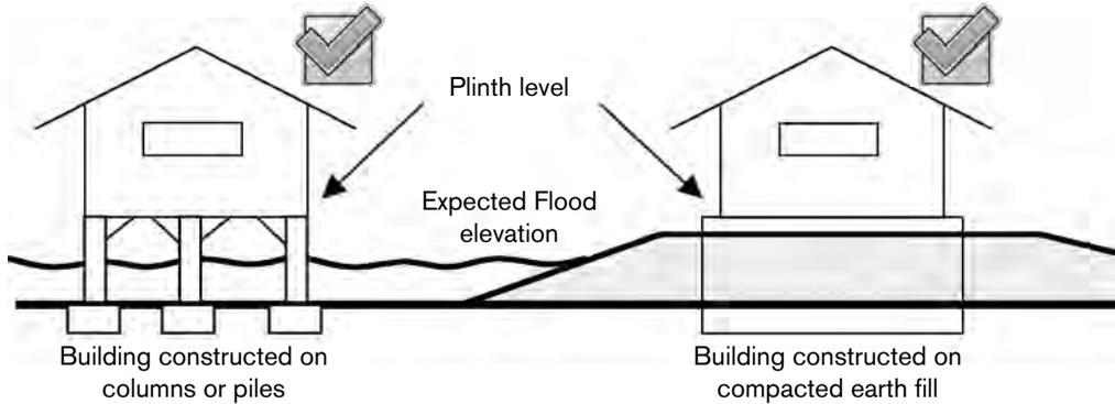
Any technique used to raise the building, must also be designed to resist the forces of standing and moving water and floating debris. Existing buildings can also be raised, although this solution can be costly and difficult. Raising masonry and concrete structures is particularly difficult and can easily damage the building.
