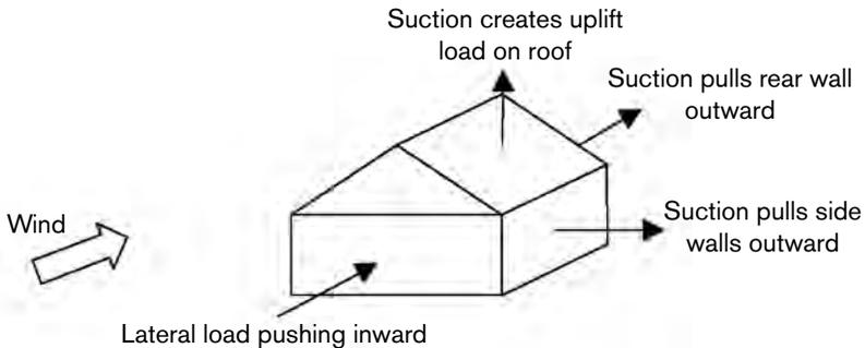
These loads may be increased or decreased based on the pressure within the building. If more air is allowed to pass through the wall facing the wind (via broken windows, severed doors, and any existing openings) the air pressure within the building will increase. This increase in air pressure inside the building will force the walls outwards. This will increase the outward pressure already exerted on the side and rear walls and roof.
