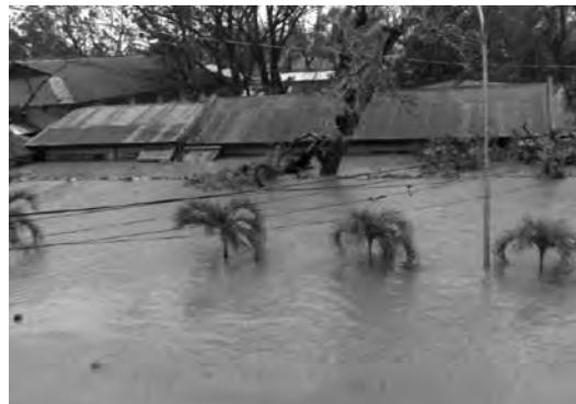
*Floods:* In the case of flooding, the selection of an adequately elevated site may eliminate a school's risk of flood damage or loss. When a suitably elevated site does not exist, modifications to the site such as adding fill to elevate the building and creating floodwalls or drainage systems can reduce potential damage and loss.
