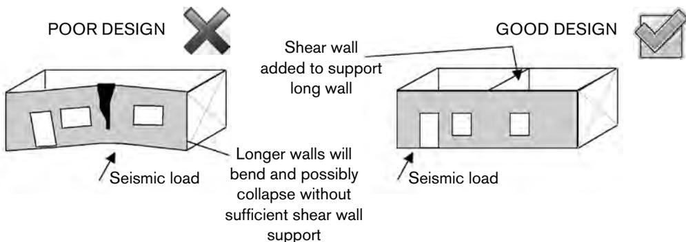
Horizontal structural components which tie all four walls together such as a floor, roof, or upper storey are called diaphragms. Diaphragms further support a face-loaded wall and transfer the load down to the shear walls, or in the case of a floor, directly to the foundation or ground.
