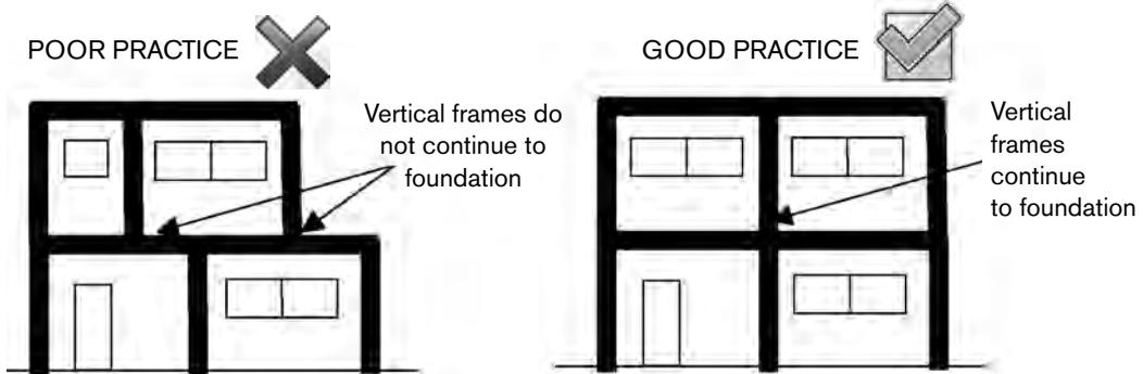
Vertical framing that does not continue to the foundation is a critical weak spot.
