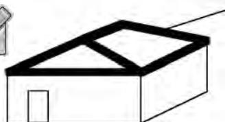
Roof perimeters and edges must resist greater uplift loads. They require reinforced connections
