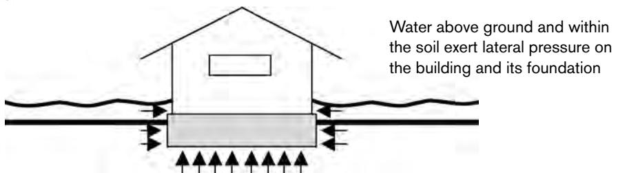
The forces of standing water (hydrostatic loads) and moving water (hydrodynamic loads) can create a very large lateral load on foundations and walls causing structural damage and collapse. See E12.
