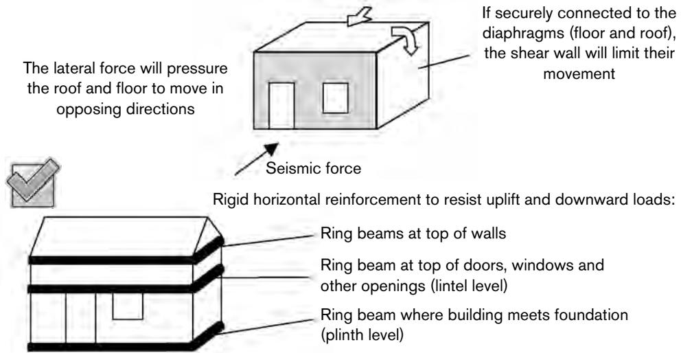
E13. To ensure that the load on a diaphragm is correctly transferred to the supporting walls, it must be rigid and act as a single element and **it must be securely attached to the walls**. An example of a rigid diaphragm would be a reinforced roof or a concrete slab floor. All walls should be securely attached to all diaphragms.
