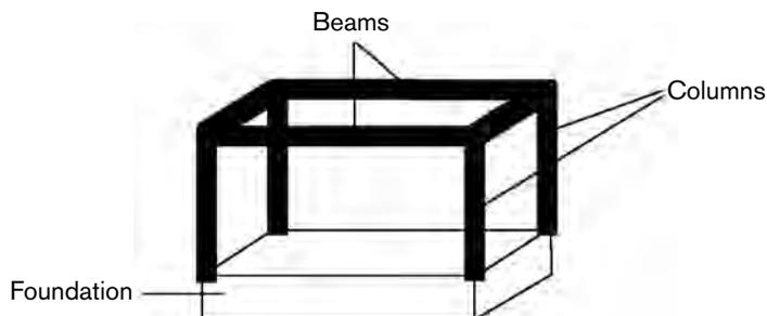
As the columns and beams joined together must resist the lateral loads, their joints must be made substantially rigid so as to maintain the box-like form. These joints are a critical point and must be securely fastened such that the joint is stronger than the structural members. Diagonal bracing can further increase the structure's lateral resistance
