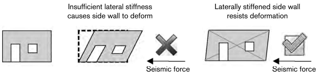
If this stiffness is insufficient relative to the load, the building will sustain damage and possibly collapse.
