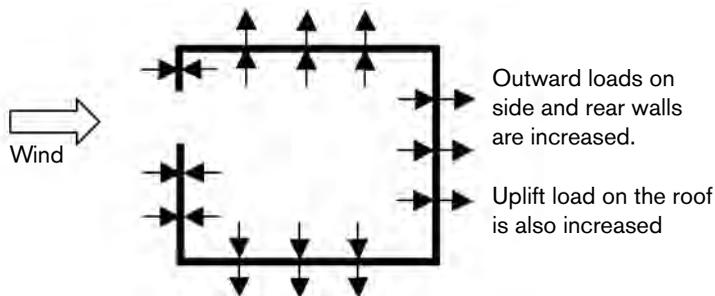
If more air is allowed to pass through the rear and side walls, the building is depressurized and air from within is sucked out of the building. This suction pressure pulls the side
