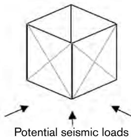
As the direction of these lateral loads cannot be predicted, the shear strength must be considered for loads from any direction. Therefore all walls should be designed to resist lateral loads.
