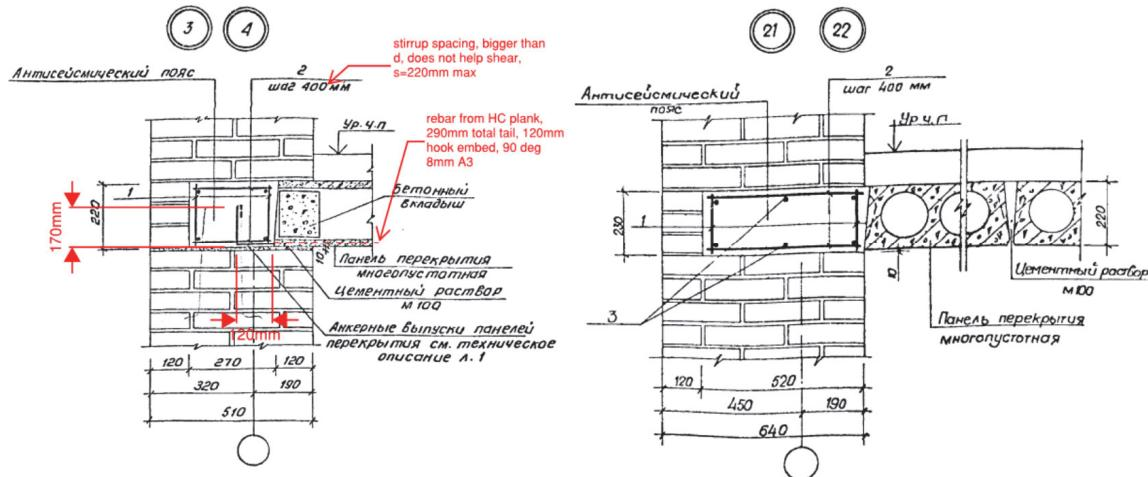
Figure 5-24 Anchorage of the structural walls.
