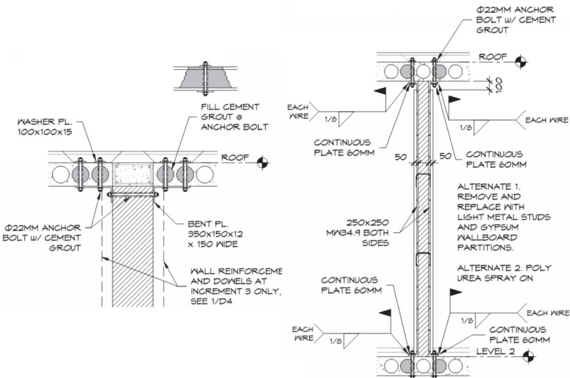
Figure 5-15 Details of CM Increment 1 showing bracing of nonstructural masonry walls.
