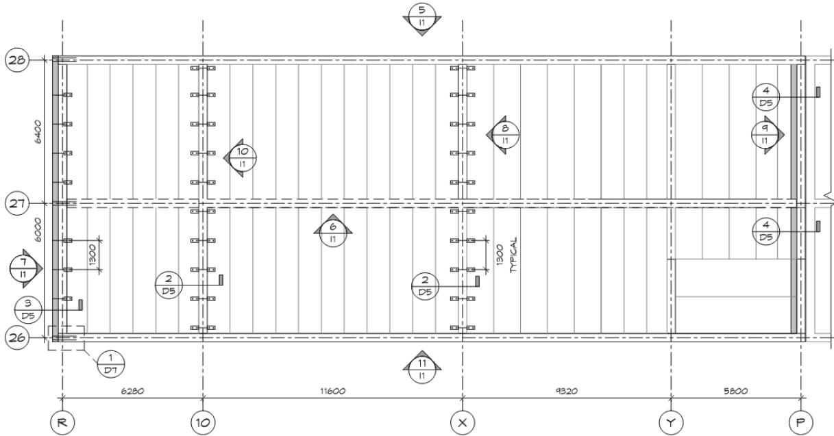
Figure 5-26 Plan showing location of transverse wall connections in CMCF Increment 1.
