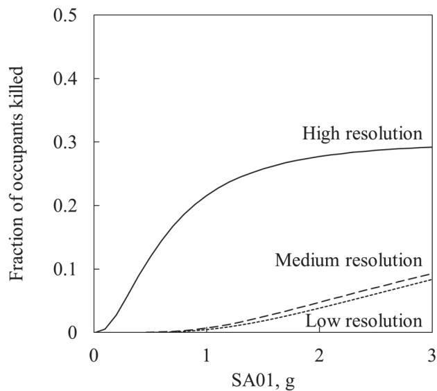
Figure H-8      Vulnerability functions for PC typology with low-, medium-, and high-resolution data. Low- and medium-resolution curves represent the equally weighted average of all buildings in the group.
