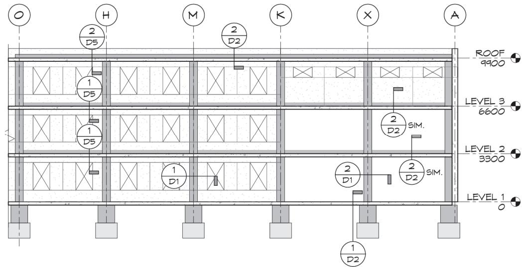
Figure 5-44 Elevation showing jacketed columns in PC Increment 2.
