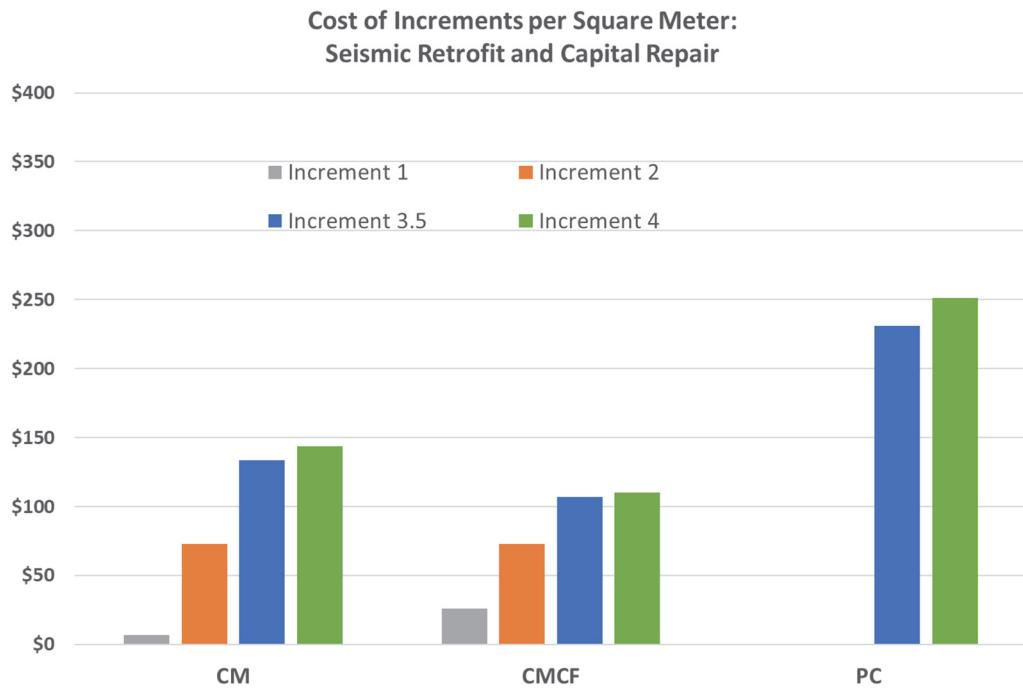
Figure 7-1 Seismic retrofit and capital repair cost estimate per square meter for three typologies at retrofit increment levels.
