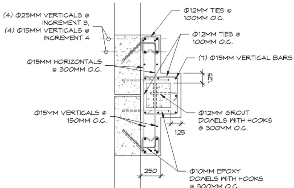
Figure 5-49 Engagement of precast panels from diaphragm in PC Increment 3.
