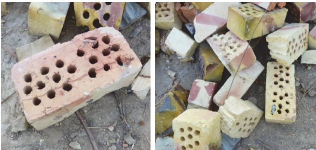
Figure 5-3 Partially fired masonry units from Kyrgyzstan (S. Brzev).
