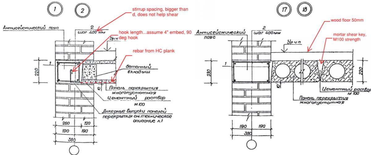
Figure 5-13 Plank to wall details. Note the positive anchorage in the load bearing direction and lack of anchorage in the non-load bearing direction.
