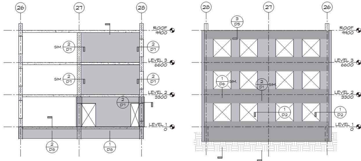
Figure 5-32 Exterior jacket of reinforced concrete in CMCF Increment 4.
