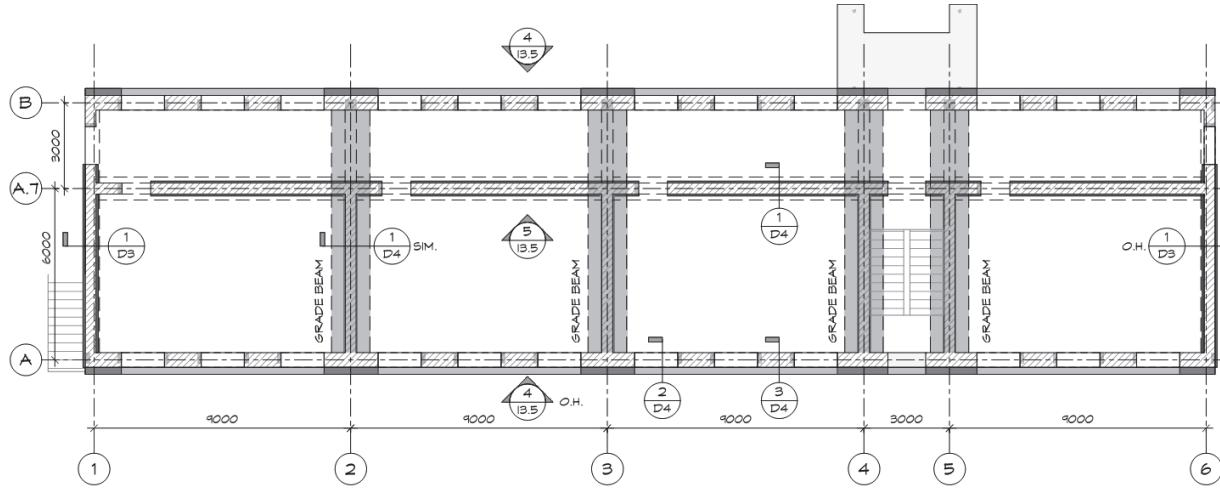
Figure 5-19 Transverse grade beams added in CM Increment 3.
