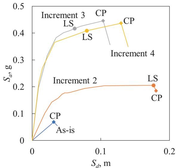
Figure 6-4 Pushover curves in the transverse direction for the precast concrete index building; one for the as-is condition, and one for each of three mitigation increments, labeled increments 2, 3, and 4. “LS” denotes a performance point at which life safety is threatened, generally by falling structural or nonstructural elements; “CP” denotes a performance point at which the building exceeds the collapse-prevention limit state.
