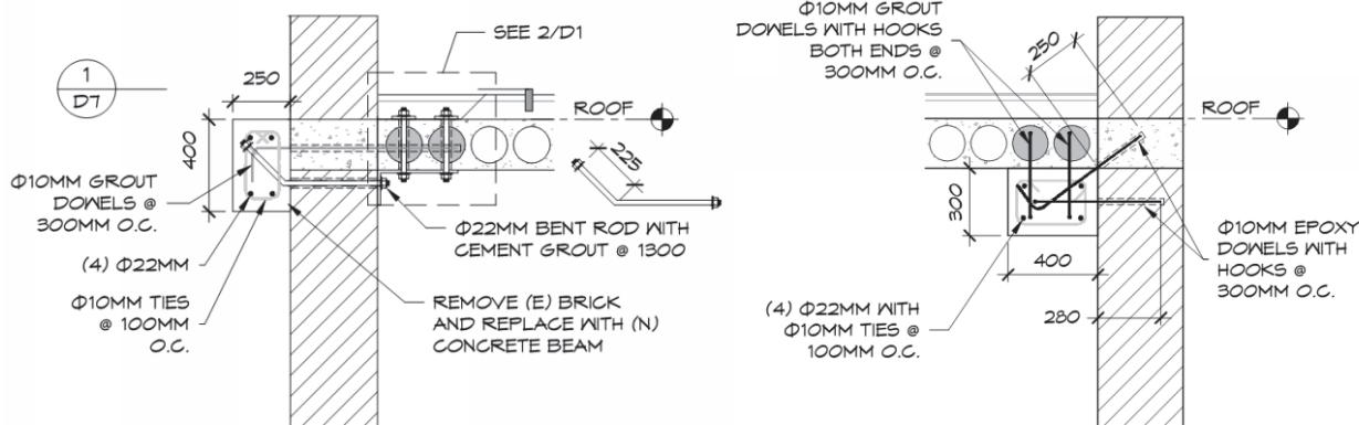
Figure 5-27 Detail of transverse wall to belt beam connection in CMCF Increment 1.
