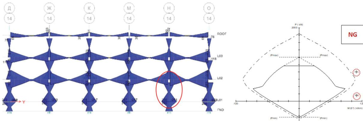
Figure 5-40 The model on the right forestalled shear failures to induce a moment demands shown. Plastic hinges form at the ground floor because the frame does not satisfy the strong column weak story criteria.
