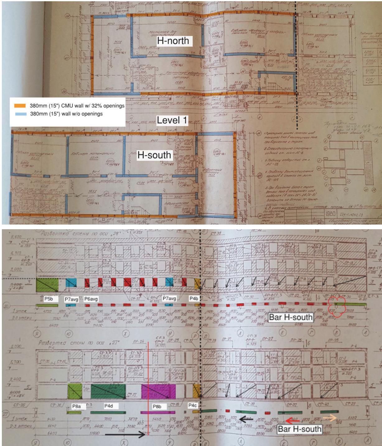
Figure 5-23 Map of structural piers and walls of CMCF index building that are assessed to determine the overall pushovers.
