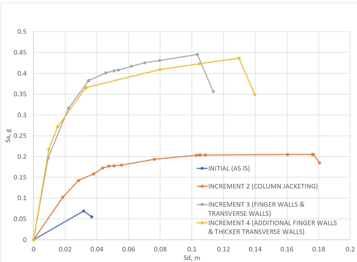
Figure 5-52 Pushover curves (spectral acceleration versus spectral displacement) for Increments 1 through 4 for PC index building, longitudinal direction.
