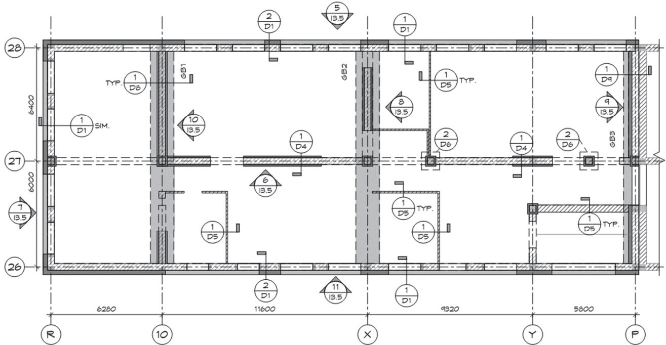
Figure 5-31 Plan showing transverse grade beams in CMCF Increment 3.5.
