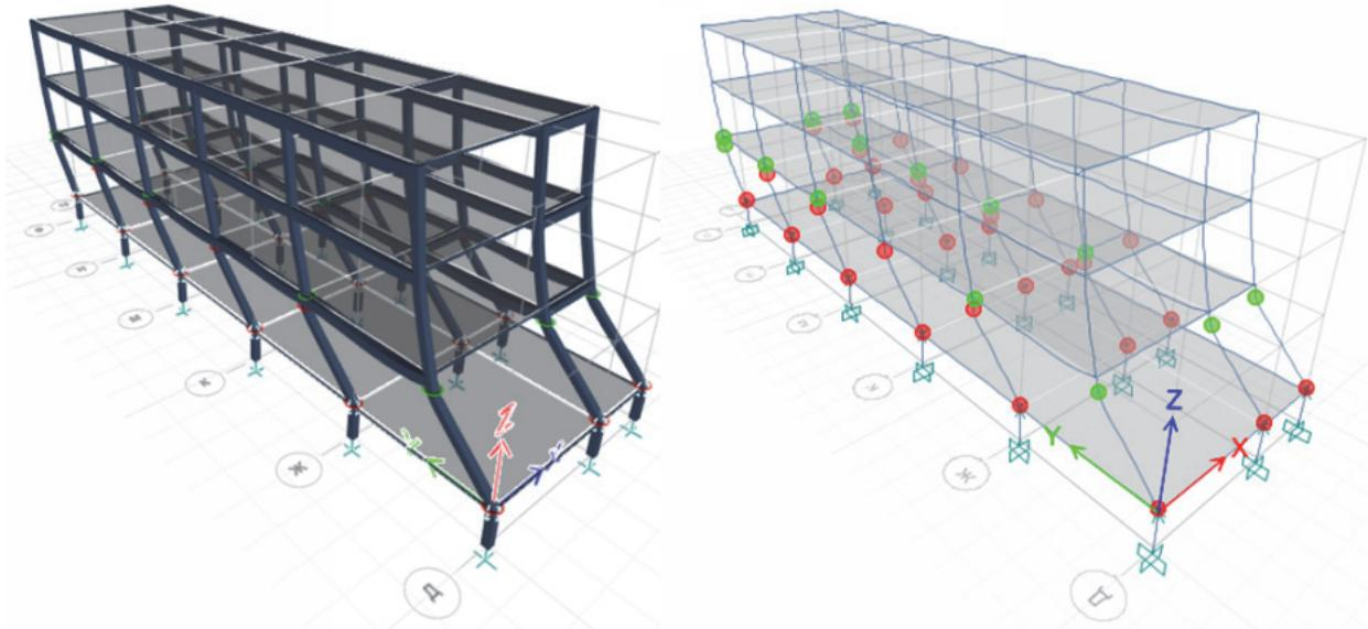
Figure 5-39 Deflected shapes of the precast frame. Shear failure was monitored and found to occur prior to flexural hinges. The model on the right forestalled shear failures to induce a side-sway mechanism at the first story. The columns are essentially fixed at the ground, due to a lock-off interaction with the slab-on-grade, and the deep footings.
