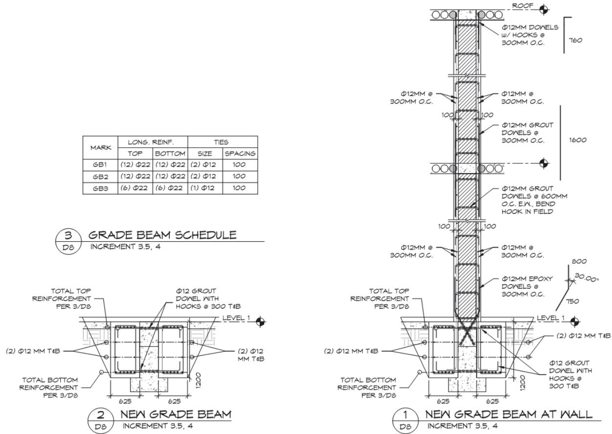
Figure 5-30 Detail of transverse grade beams in CMCF Increment 3.5.
