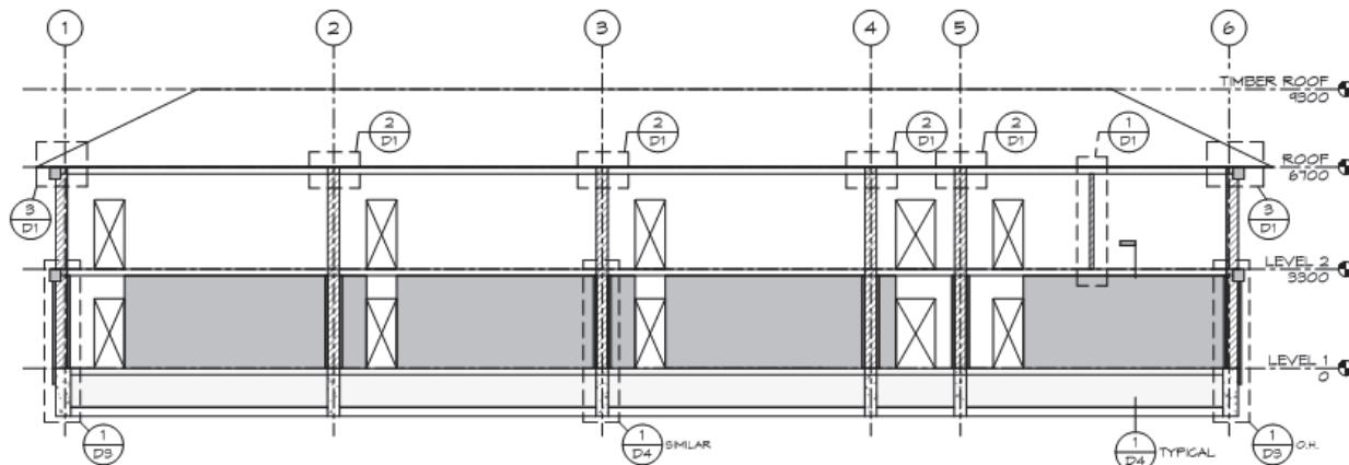
Figure 5-16      Reinforced concrete jackets added in CM Increment 2.
