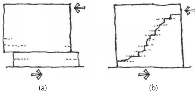
Figure 5-4 Bed joint shear and diagonal shear mechanisms.
