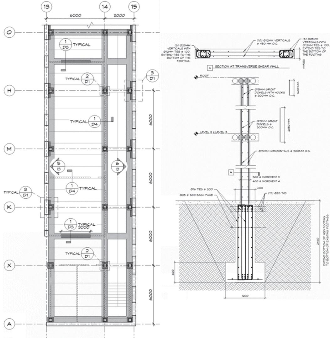
Figure 5-47 Transverse walls and foundation added for PC Increment 3.
