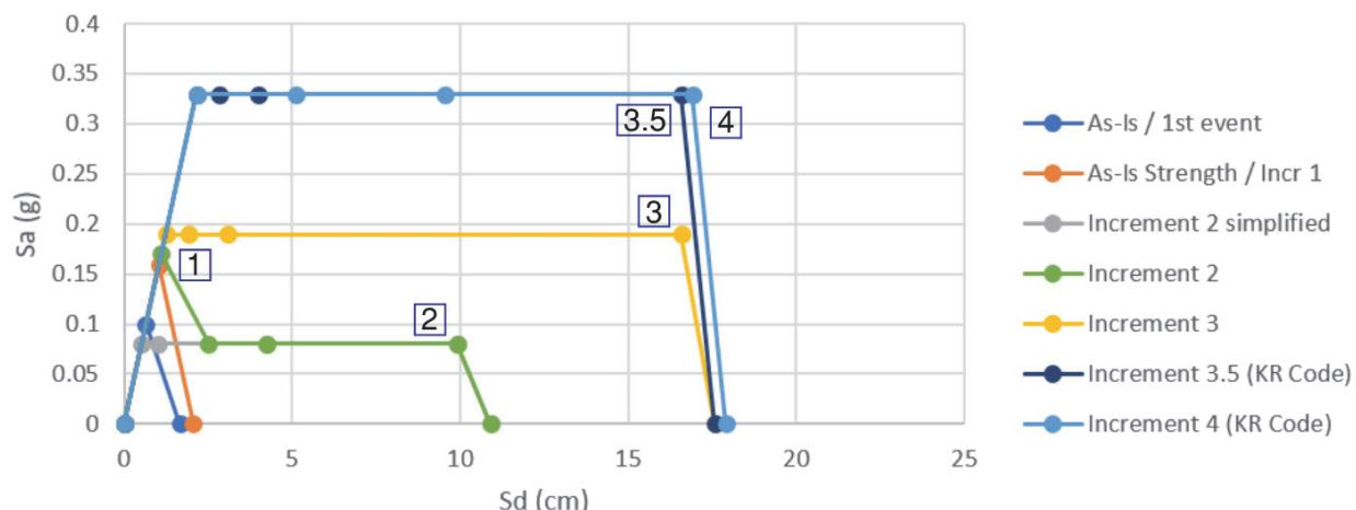
Figure 5-34 Pushover curves (spectral acceleration versus spectral displacement) for Increments 1 through 4 for CMCF index building, transverse direction.
