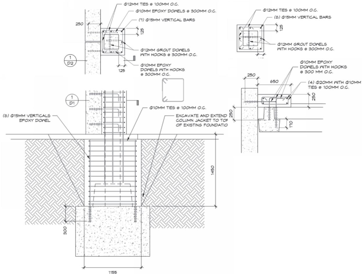
Figure 5-45 Column jackets extending to footing in PC Increment 2.
