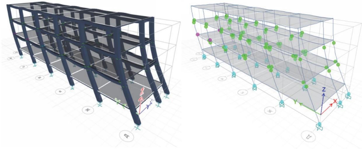
Figure 5-42 Deflected shapes of the precast frame retrofitted with reinforced column jackets. The structure is many times stronger than the as-is condition. The columns eliminate the first story mechanism.
