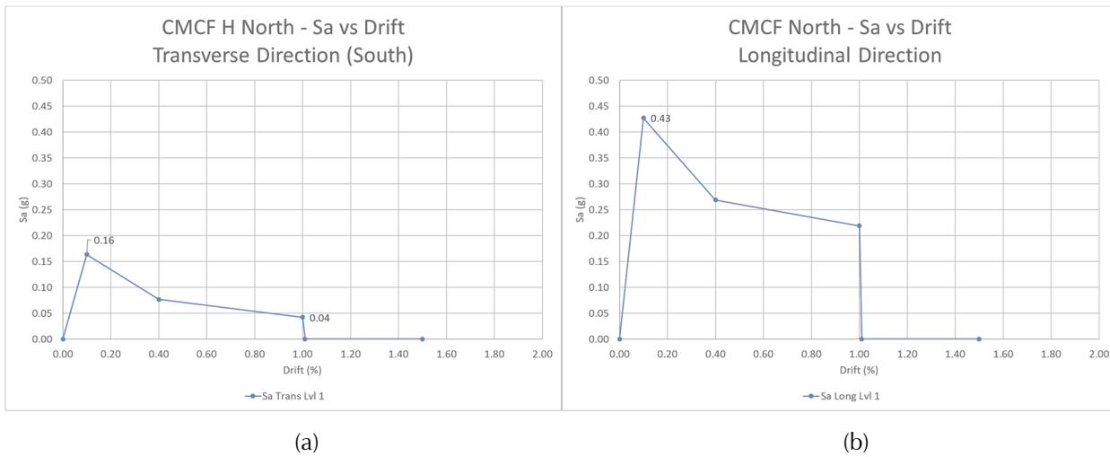
Figure 5-25 CMCF pushover curves in the as-is condition, assuming partial collapse mechanisms have been retrofitted per Increment 1: (a) transverse direction; and (b) longitudinal direction.
