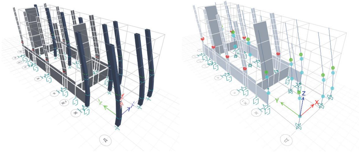
Figure 5-46 Deflected shapes of the precast frame retrofitted with Increment 3.
