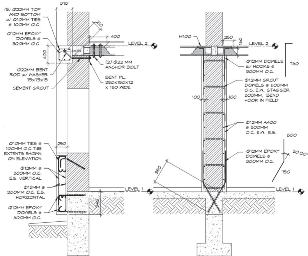
Figure 5-18 Detail of finger piers in CM Increment 2.
