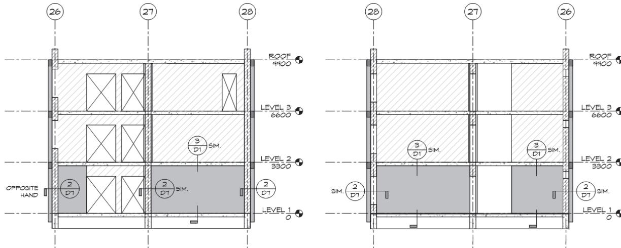
Figure 5-28 Reinforced concrete jackets added in CMCF Increment 2.
