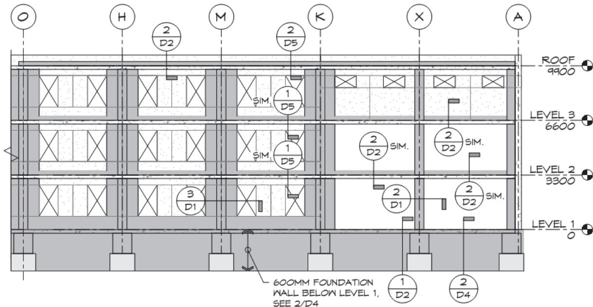
Figure 5-48 Longitudinal wall fingers added in PC Increment 3.
