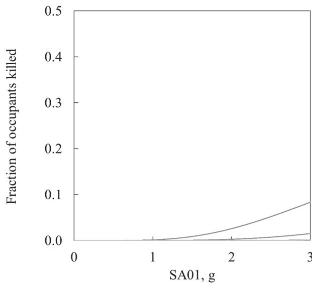
Figure H-6 Vulnerability functions for PC typology, low-resolution data.
