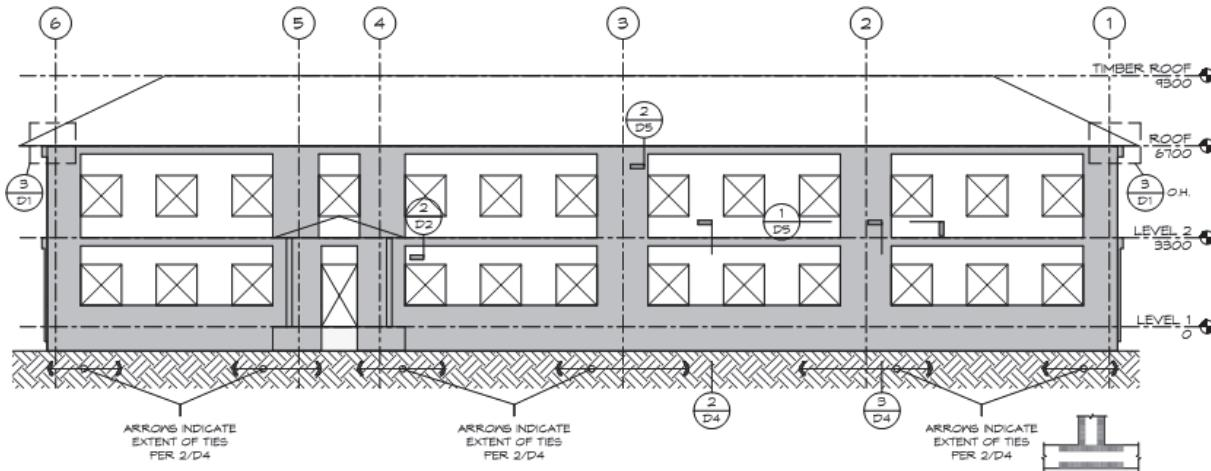
Figure 5-17 Reinforced concrete finger piers added in CM Increment 2.
