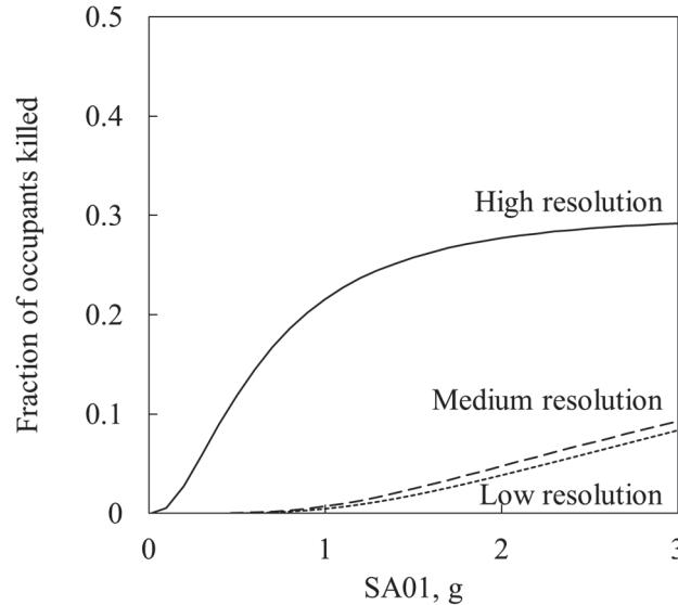
Figure 6-5      Vulnerability functions for complex masonry typology, low-, medium-, and high-resolution data.
