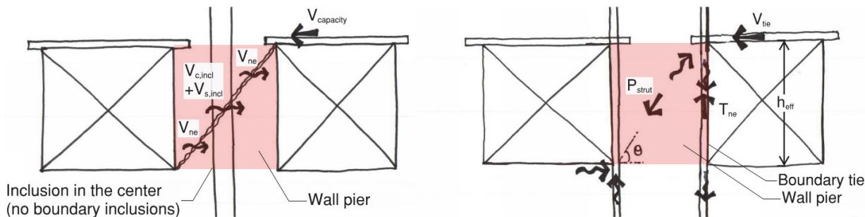
Figure 5-5 Diagonal shear mechanism with inclusions and strut-and-tie mechanism with ties from inclusions.
