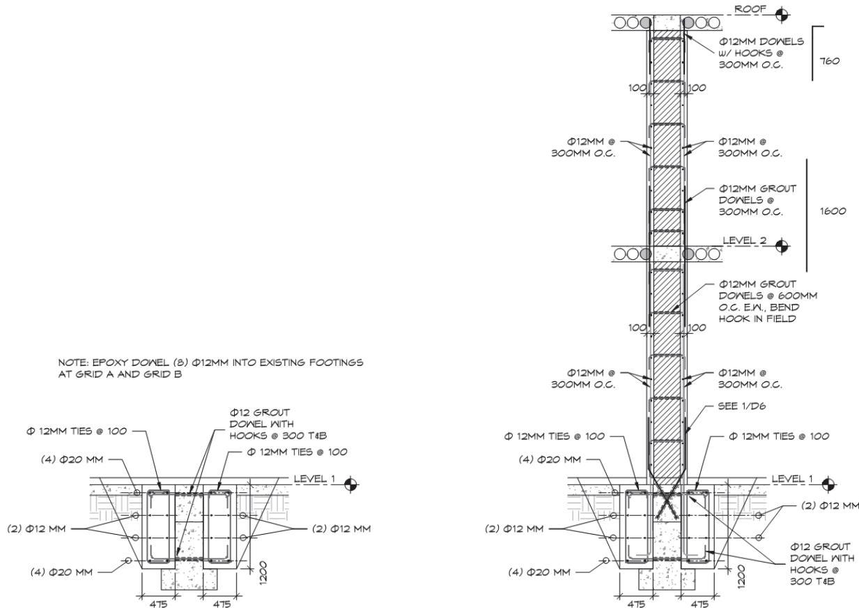
Figure 5-20 Detail of transverse grade beam in CM Increment 3.
