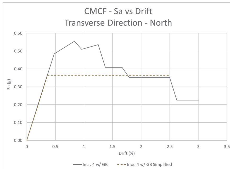
Figure 5-33 Pushover curves (spectral acceleration vs. spectral displacement) for CMCF Increment 4, transverse direction. The irregular shape is due to the degrading response of the grade beams, per the backbone curves of ASCE/SEI 41-17. The dashed line shows the simplified version that was used for the benefit cost analysis.
