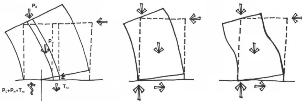
Figure 5-6 Flexure with toe crushing and flexure with rocking mechanisms.
