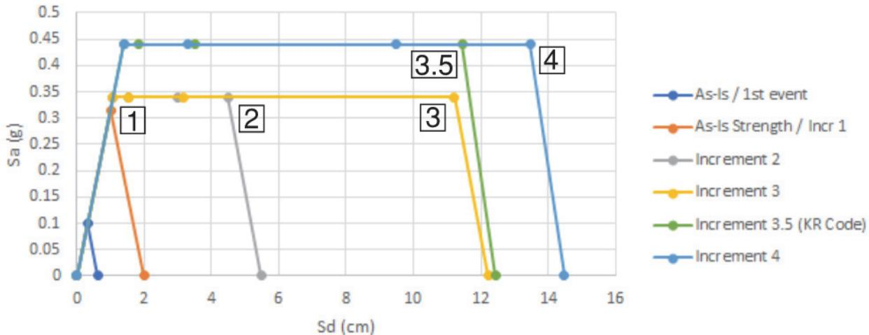
Figure 5-22     Pushover curves (spectral acceleration versus spectral displacement) for Increments 1 through 4 for CM index building, transverse direction.
