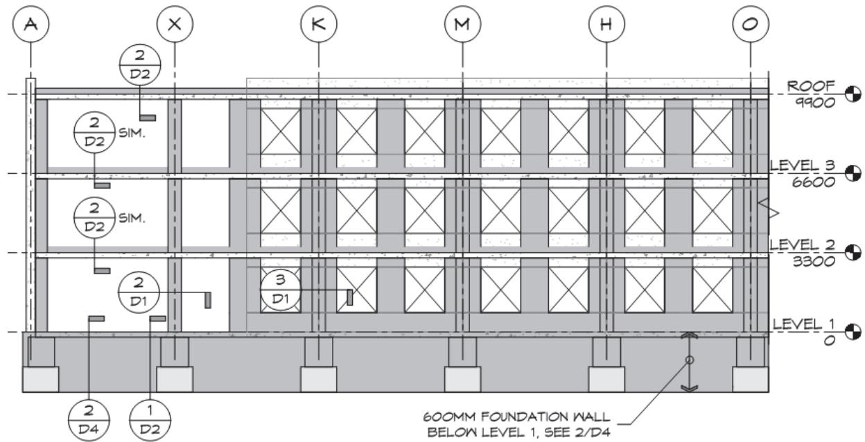
Figure 5-50 Reinforced concrete fingers covering every precast panel in PC Increment 4.
