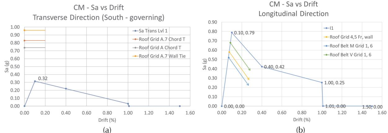
Figure 5-14 CM pushover curves in the as-is condition, assuming partial collapse mechanisms have been retrofitted per Increment 1: (a) transverse direction; and (b) longitudinal direction. The curves for each direction are the summation of the backbone curves for the individual piers.
