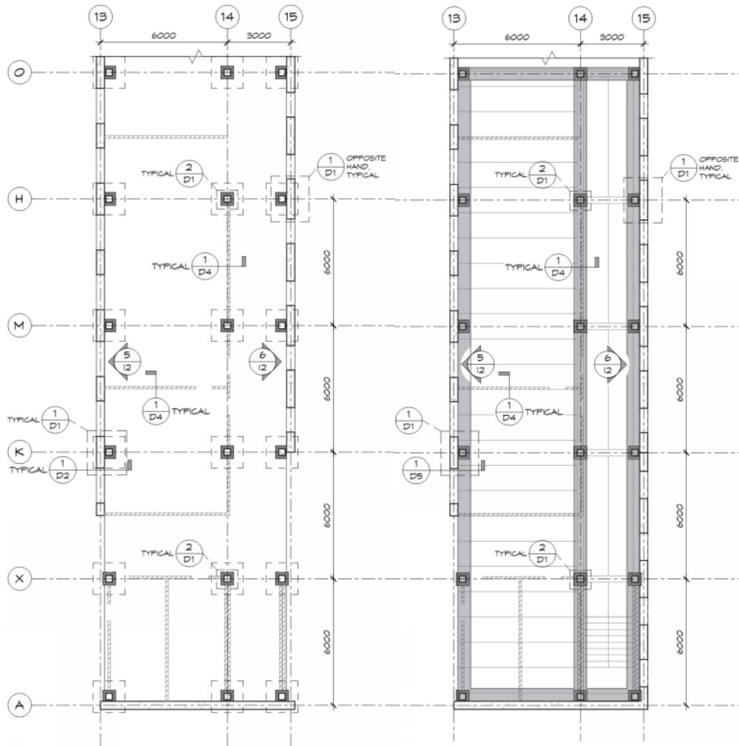
Figure 5-43 Plan showing columns and nonstructural walls with jacketing in PC Increment 2.
