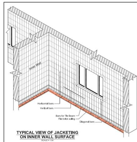
Inner surface reinforcement details
