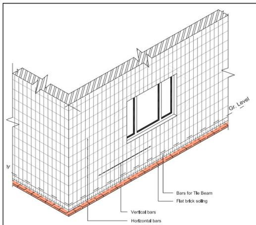
Outer surface reinforcement details
