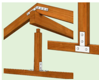
Illustration of improvement of joints in timber roof structures using straps and nails. (Reproduced from NRA, 2017).
